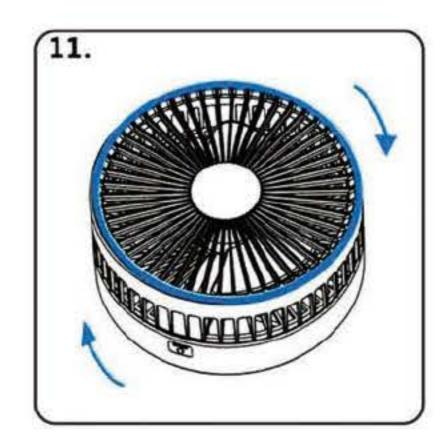
After the mask is left to dry, align the buckle and put it back in clockwise
