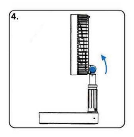
The fan can adjust the wind direction 180° up and down
