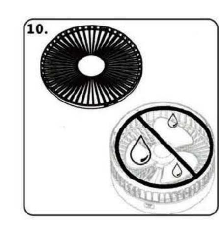
The mask can be removed to clean the dust.
