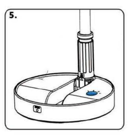
Single-click the switch to display the power level double-click the switch to turn on the fan to adjust the wind speed at level 1, 2, and 3 long-press for 2 seconds at level 4 to shut down
