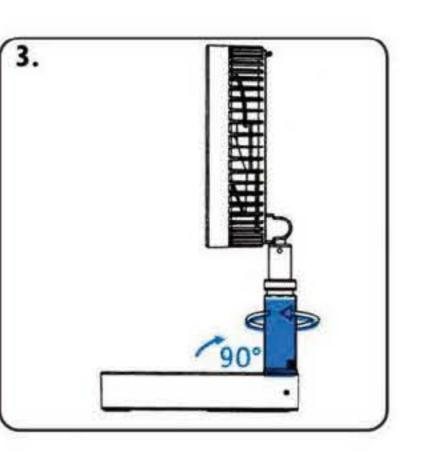
After turning on the fan adjust the angle to 90° vertically and then tightenthe handle clockwise to fix the angle
