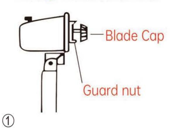
Put rear grill on motor shaft and secure with guard nut.
