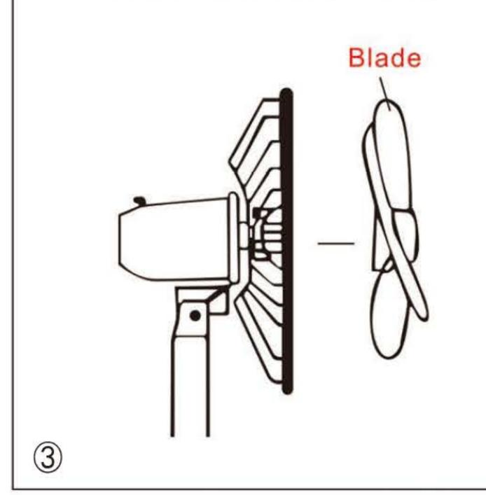
Screw blade cap on shaft by turning counter clockwise.
