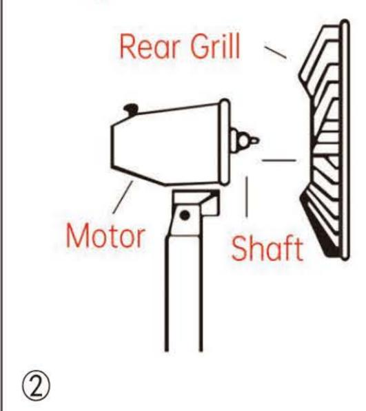
Slide blade on motor shaft.
